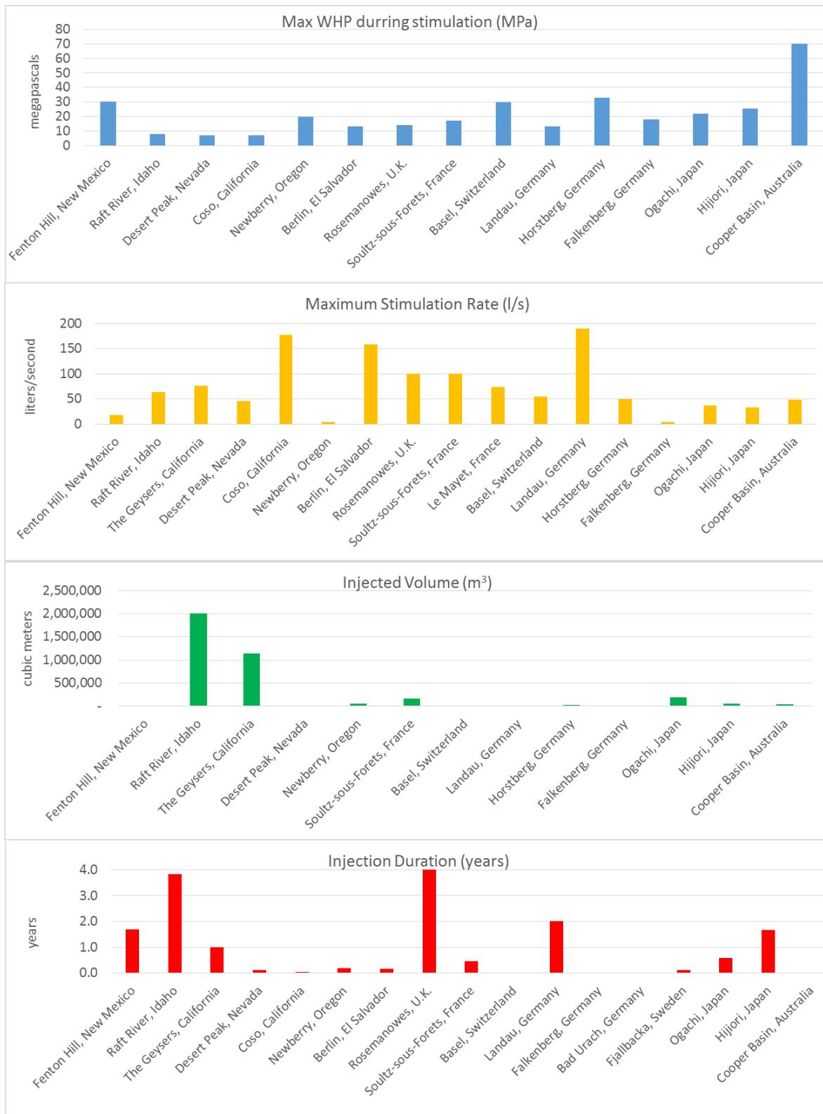
Figure 9: Maximum well head pressure (WHP), maximum flow rates, injected volume and injection duration by EGS site as reported in the literature.
