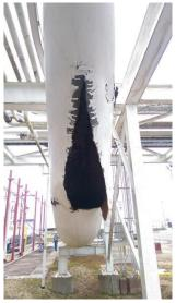
Figure 24: Big Hill SPR Site Raw Water Header Piping Failure April 2016
