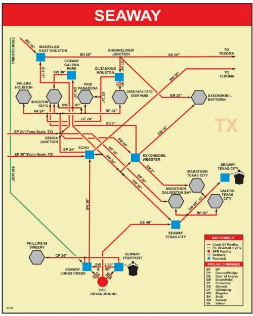
Figure 12: Seaway System Diagram
