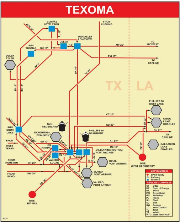
Figure 13: Texoma System Diagram
