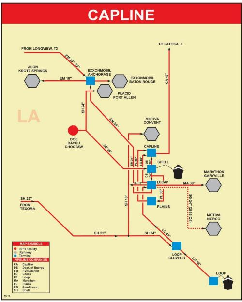
Figure 14: Capline System Diagram
