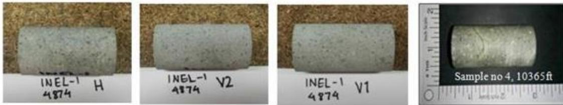
Figure 7: Pictures of samples before the triaxial or injection tests
