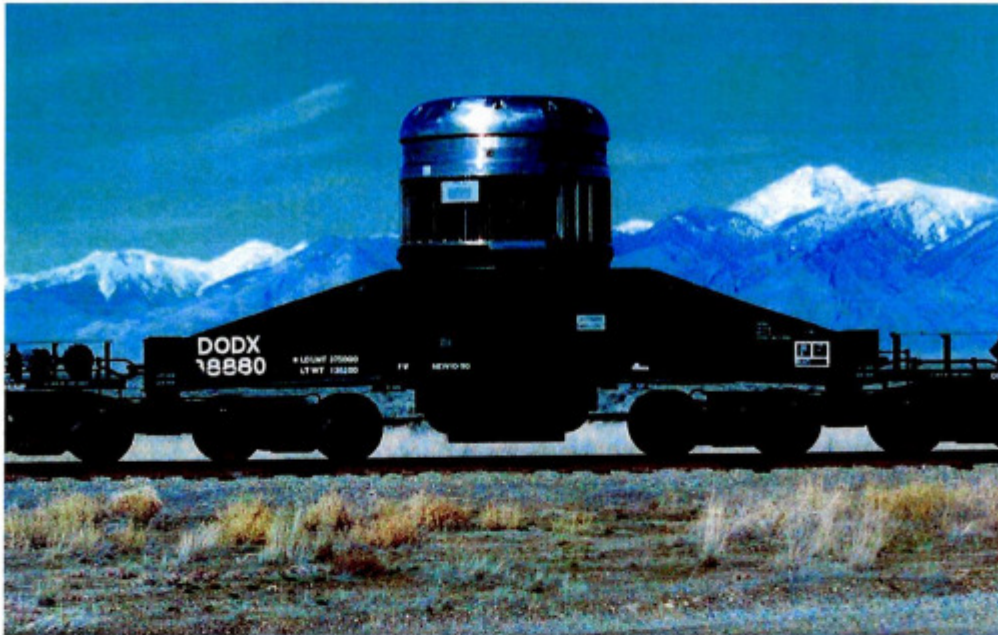
Figure 2: M-140 Shipping Container
