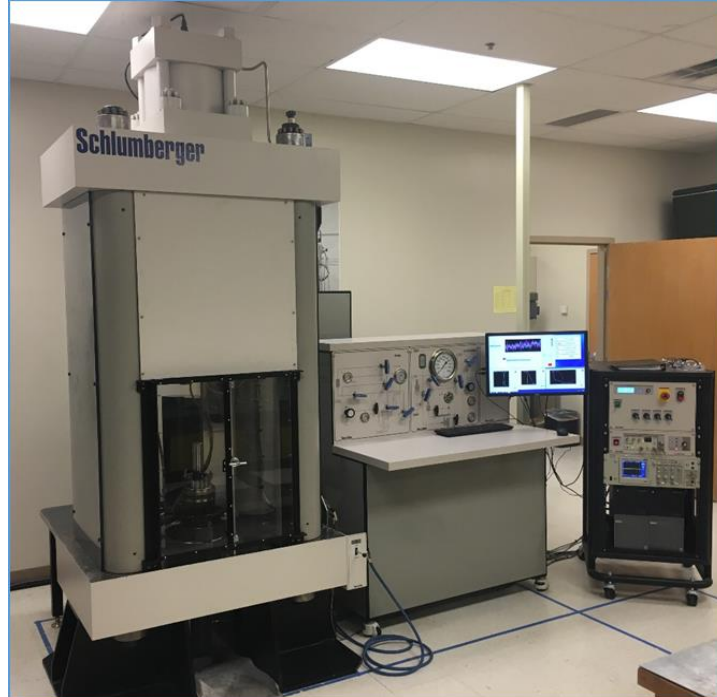
Figure II: Triaxial compression loading frame use to measure the mechanical properties described subsequently.
