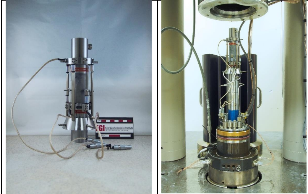
Figure 2: The left hand panel shows a sample encapsulated in a shrink-fit Teflon jacket to prevent penetration of confining fluid. These measurements were made at ambient temperature. Also visible are cantilever devices to determine average axial strain and radial strain in two orthogonal directions. The panel at right shows the same sample configuration mounted on a base plug and a load cell, immediately before being raised into the confining pressure vessel (at top of photograph) prior to testing.
