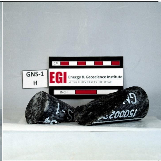
Figure 3b. This is a post-test view of sample GNS-1H. The H designates an orientation normal to the axis of the core (horizontal).
