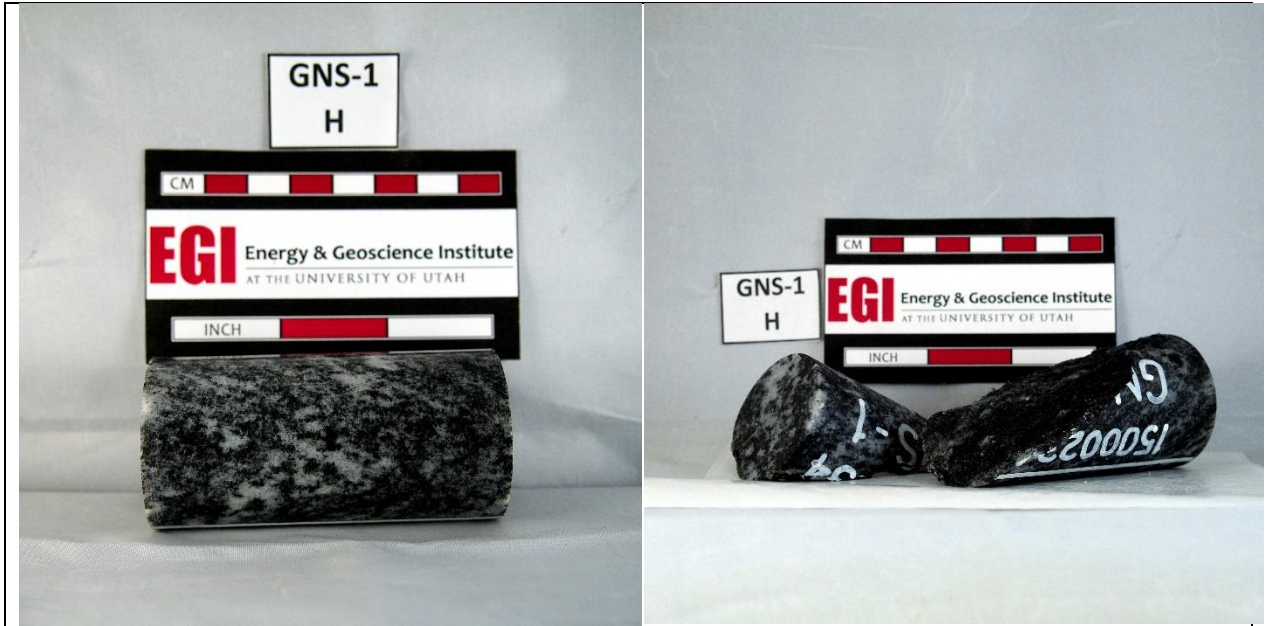
Figure 13a. This is a pre-test view of sample GNS-1H. The H designates an orientation normal to the axis of the core (horizontal).
