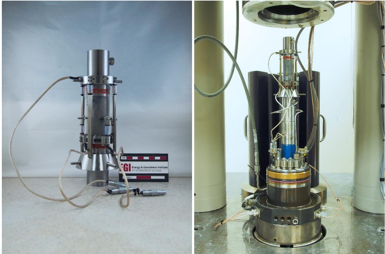
Figure 35: The left hand panel shows a sample encapsulated in a shrink-fit Teflon jacket to prevent penetration of confining fluid. These measurements were made at ambient temperature. Also visible are cantilever devices to determine average axial strain and radial strain in two orthogonal directions. The panel at right shows the same sample configuration mounted on a base plug and a load cell, immediately before being raised into the confining pressure vessel (at top of photograph) prior to testing.
