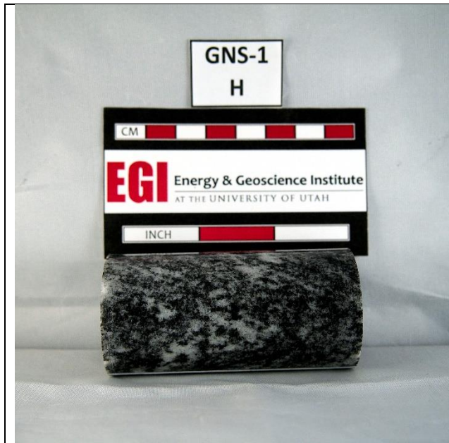
Figure 3a. This is a pre-test view of sample GNS-1H. The H designates an orientation normal to the axis of the core (horizontal).
