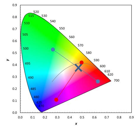
Figure 2. Chromaticity diagrams, such as the CIE 1931(x, y) chromaticity diagram shown here, are used to provide a numerical specification for the color of light. The colored background is for visual reference only, as chromaticity diagrams do not account for lightness. The numbers around the outside indicate the wavelength of monochromatic light at the coordinate, in nanometers. Colors outside the shaded area are not visible to humans.
