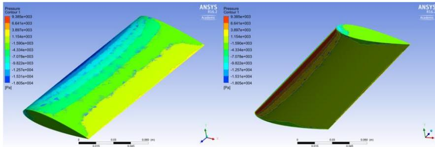
Figure 17. Aerodynamic Pressure NACA 0018 Blade
