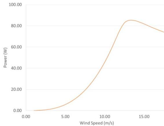
Figure 25. Power Curve for Scale Model without electrical system
