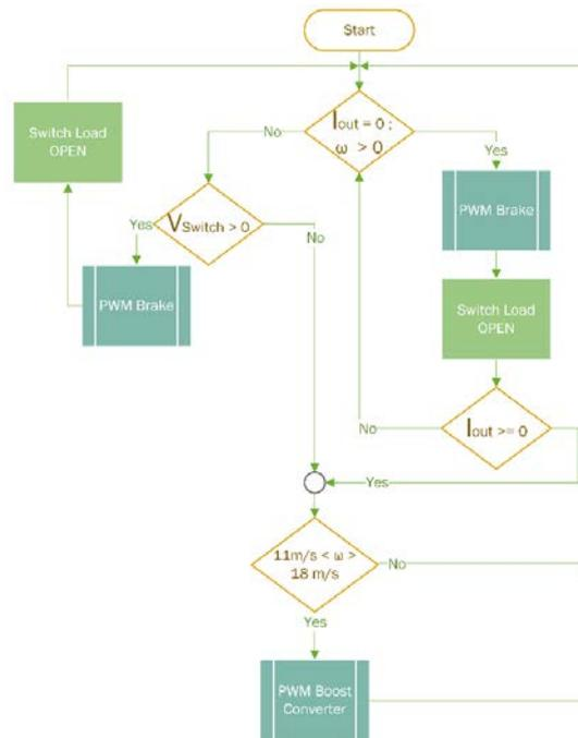
Figure 31. Flowchart for rated speed control and braking
