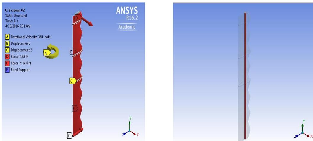
Figure 26. Blade with internal rod
