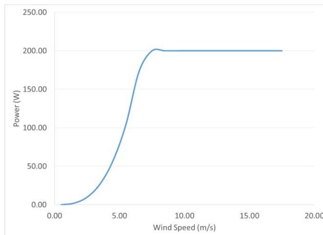
Figure 22: Power Curve of modified Whale Turbine
