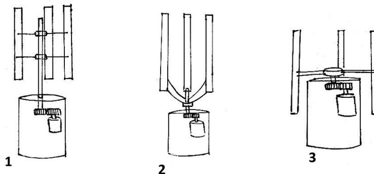
Figure 12. From left to right, rotor assembly configuration alternatives 1, 2 & 3
