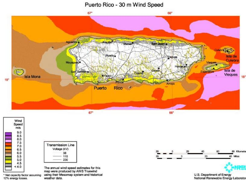
Figure 35. Wind speed map at 30m [27]
