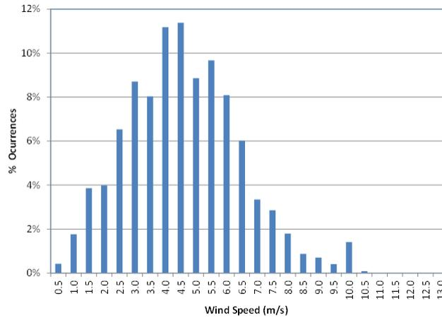
Figure 23. Histogram for wind data at Fajardo, PR [26]
