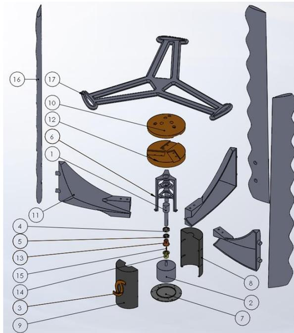
Figure 24. Final System Assembly
