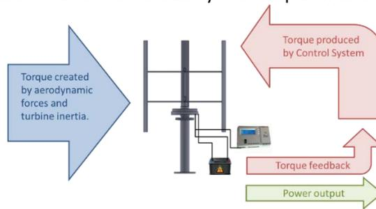
Figure 13. Interface Requirements for the Electrical & Controls Sub-System
