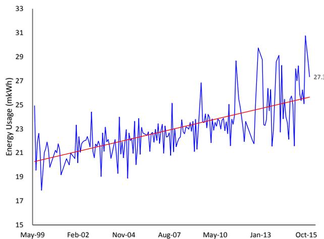
Figure 3. Monthly energy consumption for public illumination in PR [7]
