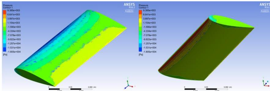
Figure 17. Aerodynamic Pressure NACA 0018 Blade
