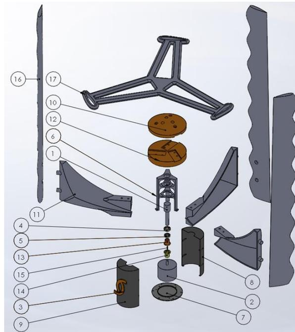
Figure 24. Final System Assembly
