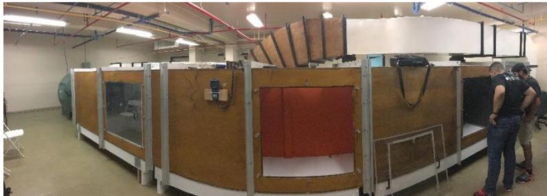
Figure 33. Close-Loop Wind Tunnel at the University of Puerto Rico, Cayey Campus
