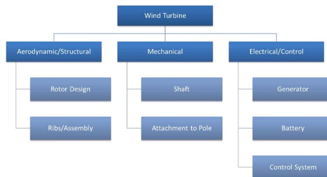
Figure 9. Wind Turbine Product Breakdown Structure diagram
