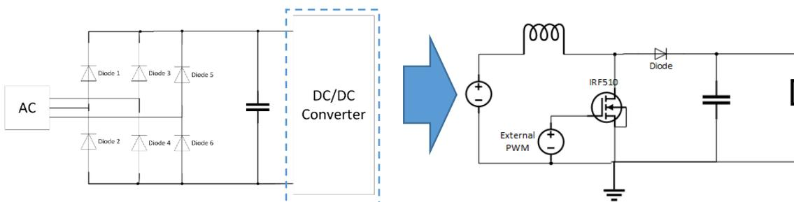
Figure 30. Three phase rectifier circuit and DC/DC boost converter
