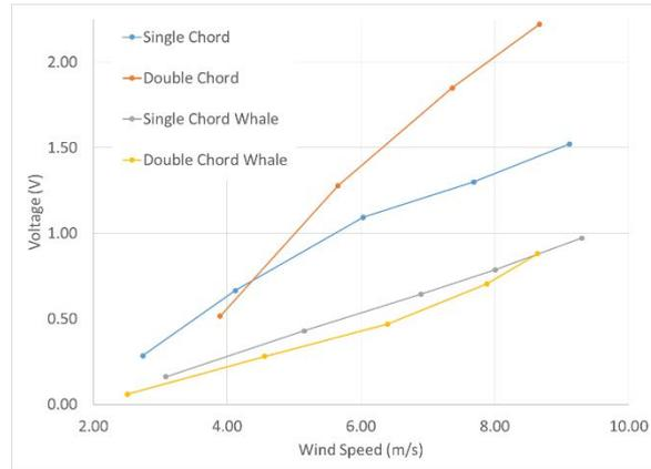
Figure 32. Voltage vs. Wind Speed data collected from preliminary tunnel testing of 2.4:1 model with scoop
