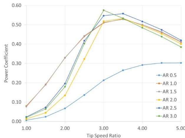
Figure 11.  $C_p$  and TSR curves comparison for all six VAWT concepts
