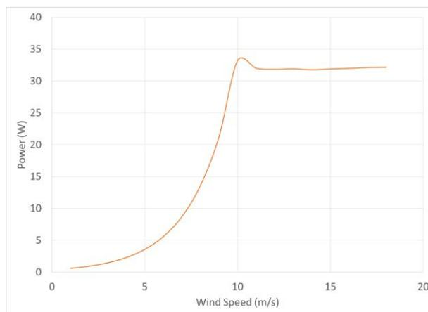
Figure 34. Wind speed vs Power output using 30W load
