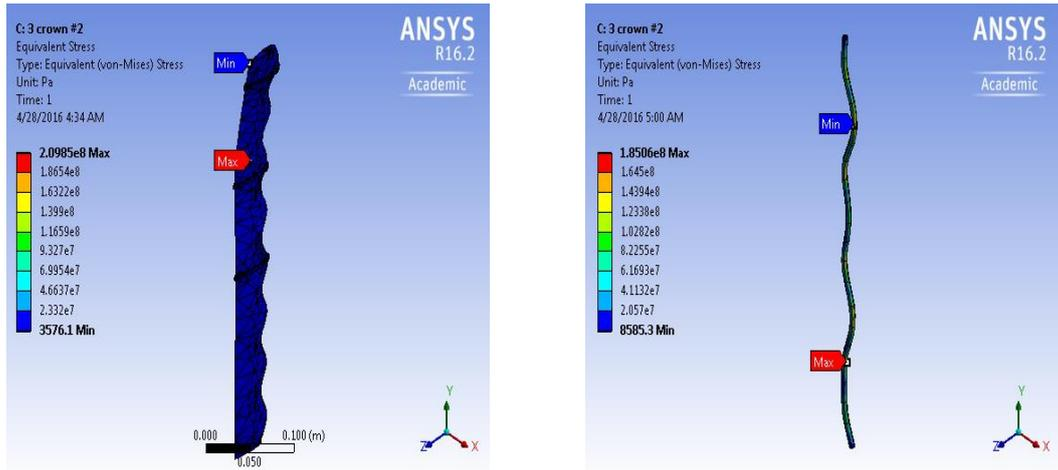
Figure 27. Scale blade structural analysis results
