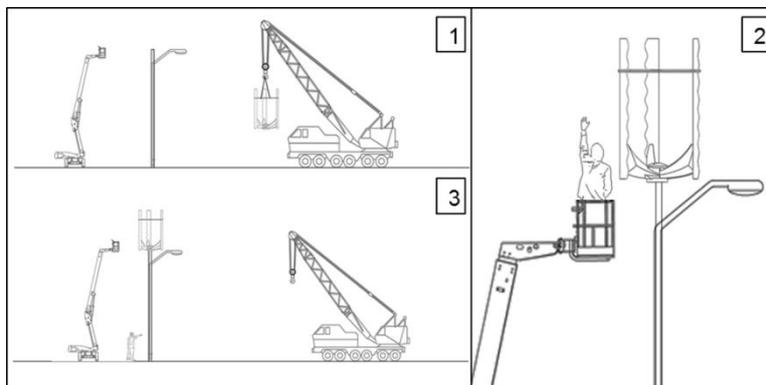
Figure 39. Process of installation to existing light pole
