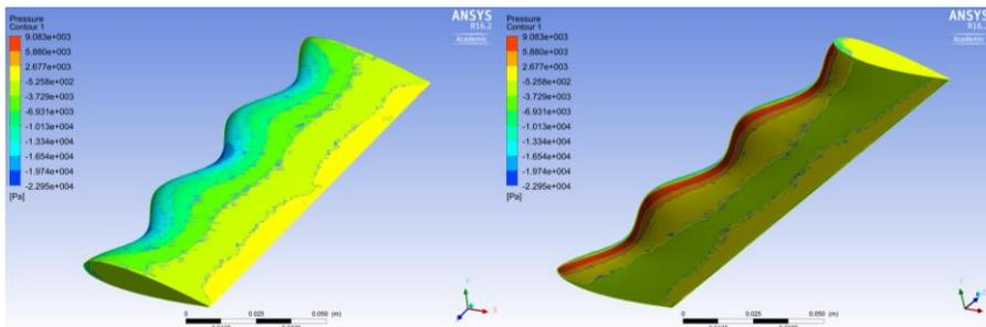
Figure 18. Aerodynamic Pressure NACA 0018 Whale Blade
