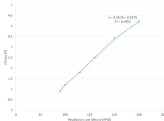
Figure 28. Voltage vs. RPM Micro-Wind Turbine Generator
