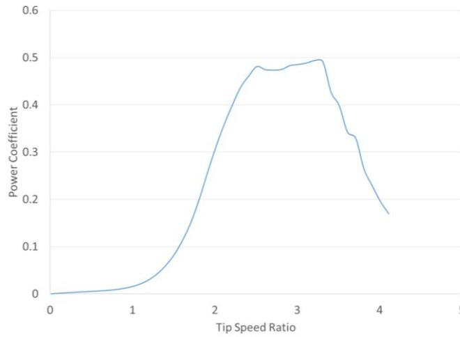
Figure 16.  $C_p$  vs. TSR for optimize turbine rotor
