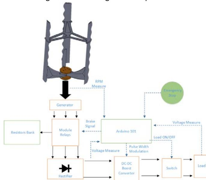
Figure 29. Electrical and Control System Diagram
