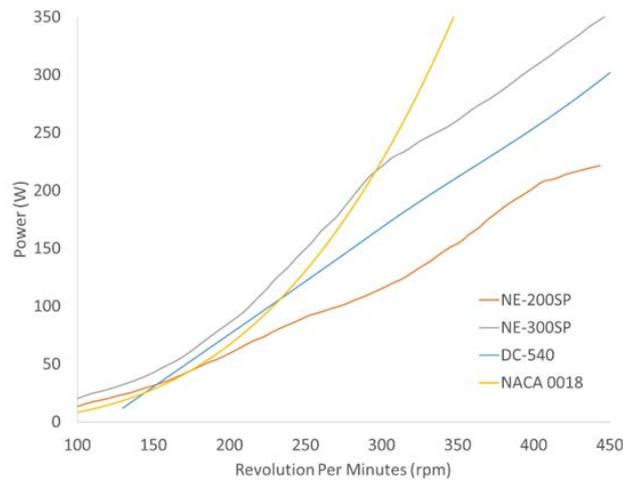
Figure 15. Power Curves for the generator comparison
