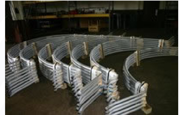
Spray coated boiler tubes www.asbindustries.com
