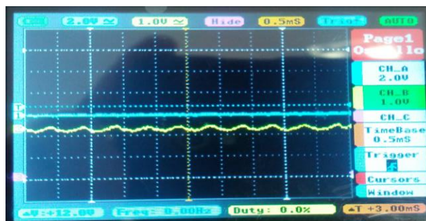
Figure 2-7: Rectifier DC Output w/ a Capacitor ( \Delta x = 0.5 \text{ ms} , \Delta y = 1V )
