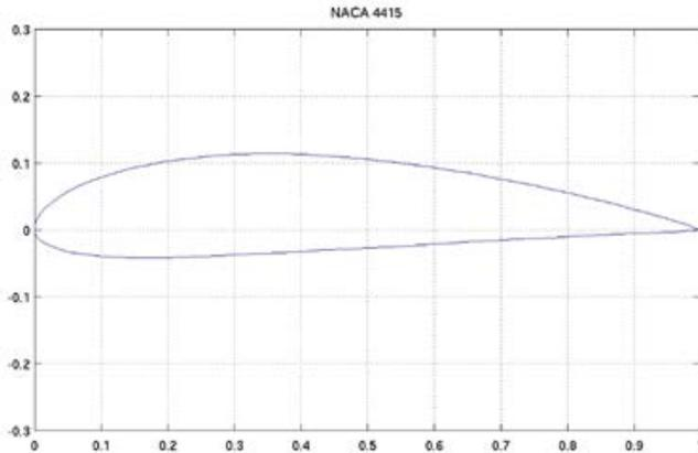
Figure 10: NACA 4415 Airfoil
