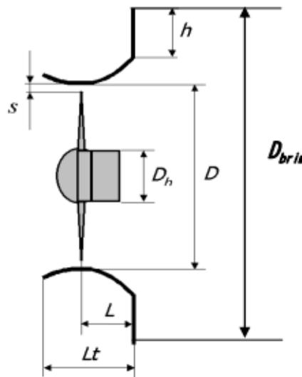
Figure 6: Wind Lens Components
