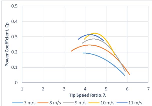
Figure 14:  $C_p$  vs. TSR – Without Wind Lens
