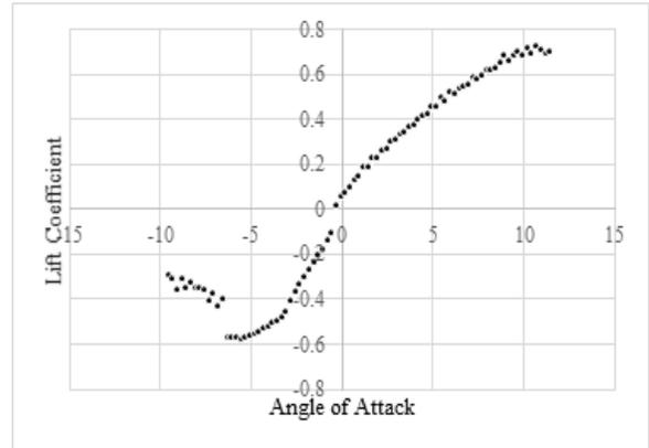
Figure 11: Prototype Lift Coefficient vs. Angle of Attack
