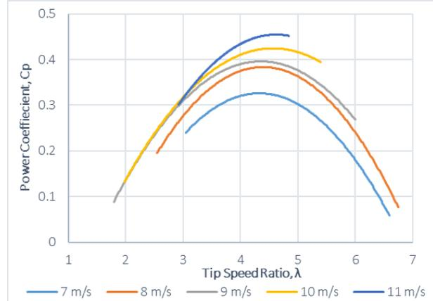
Figure 15:  $C_p$  vs. TSR - Wind Lens Added
