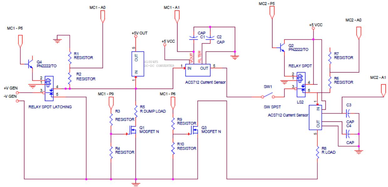
Figure 12: Electrical One-Line Diagram of Turbine System Connected to Load System
