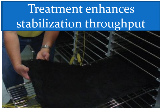
Lignin mat after stabilization
