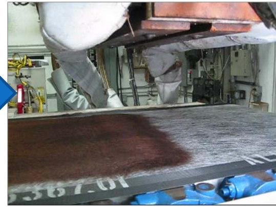
Lignin fiber mat by melt processing
