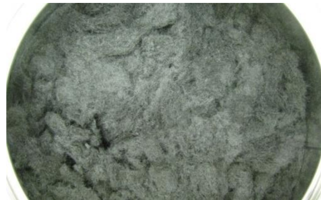
Lignin fiber after carbonization and milling
