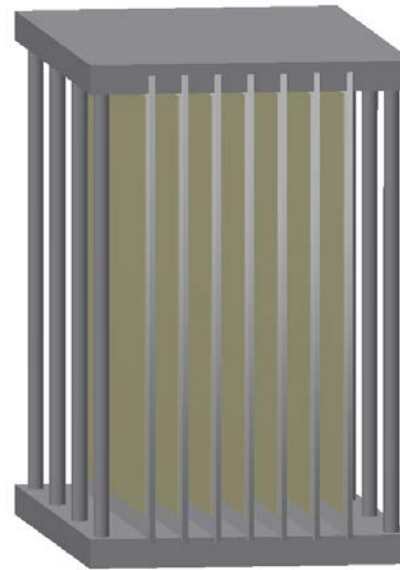
Initial fixture designed with a 5 mm spacing to ensure no depletion of reactant gasses
