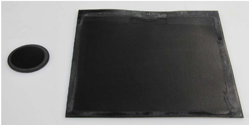
Scaled to 2 sided large area electrodes 81 cm 2 per side
