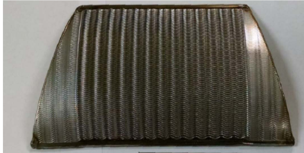
Folded, crushed and welded AFA 80 \mu m foil air cell
