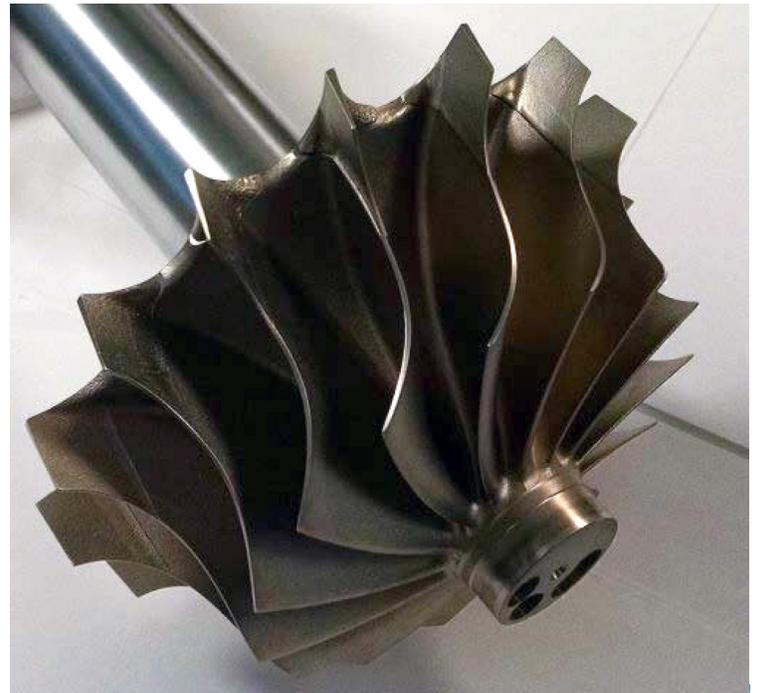
A prototype of a bi-metallic turbine wheel for the C370. The design is based on the C65 turbine wheel, but the C370 requires a stronger material due to higher temperatures and speed.
