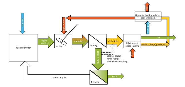
Figure 6.2. Process concept for extraction of oil from algae with a secondary amine solvent. This is followed by CO<sub>2</sub>-induced phase splitting for solvent recovery and N<sub>2</sub>-induced backswitching (Source: Du et al. 2013).
