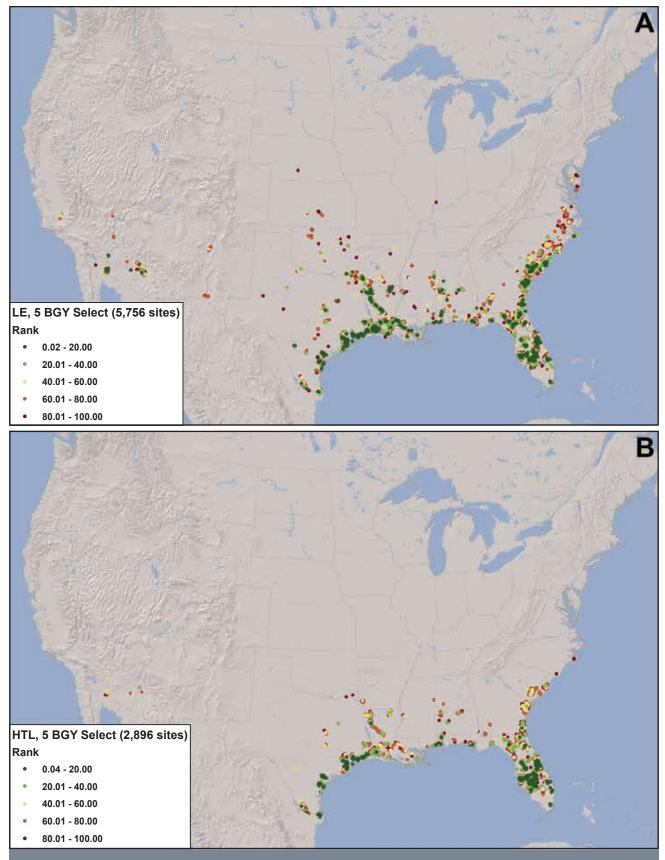
Figure 10.5. Examples of the preferred geographic regions for algal biomass production. Map showing 5 BGY site selections for LE (*A*) and HTL (*B*) scenarios. The sites are colored according to decimal rank, with the most cost-effective sites (selected first) having small numbers (and colored green). (Source: Venteris et al. 2014a)
