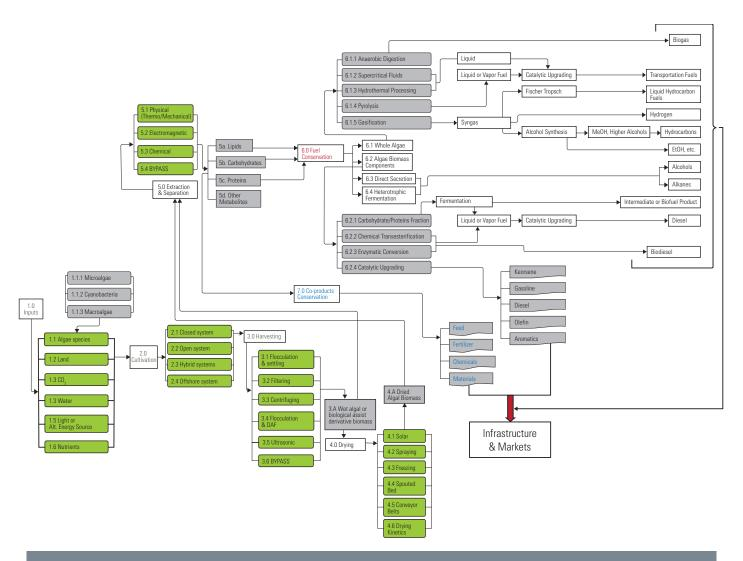
Figure 11.3. High-level multi-pathway algae biofuel process flow diagram for the algal biofuels and co-products supply chain. (Source: Adapted from the 2010 *National Algal Biofuels Technology Roadmap*.)
