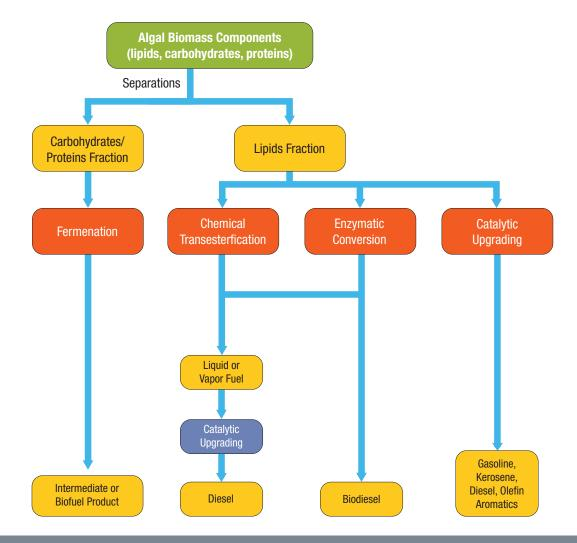
Figure 7.3. Schematic of the various conversion routes for algal biomass components into biofuels (Source: Adapted from the 2010 *National Algal Biofuels Technology Roadmap.*)
