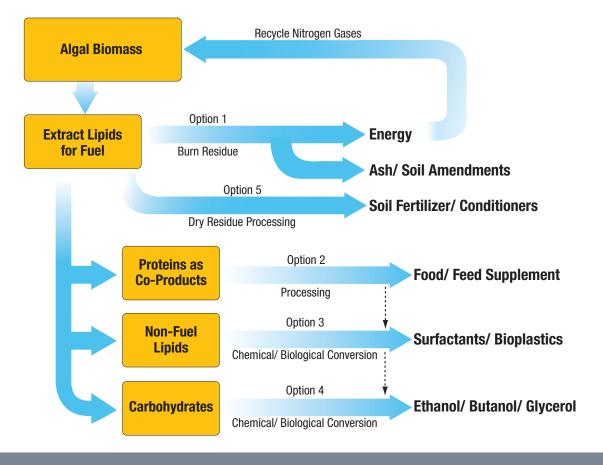
Figure 8.2. Overview of the five potential options for the recovery and use of co-products
