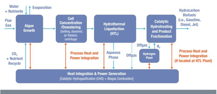
Figure 11.5. AHTL process flow diagram (Source: DOE 2016)
