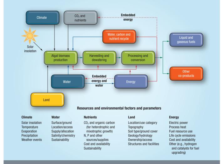
Figure 10.1. High-level overview of the algal biofuel supply chain, illustrating key resource inputs and related environmental issues spanning the operations of biomass production through downstream processing and conversion to fuels and co-products. (Source: From Pate 2013)
