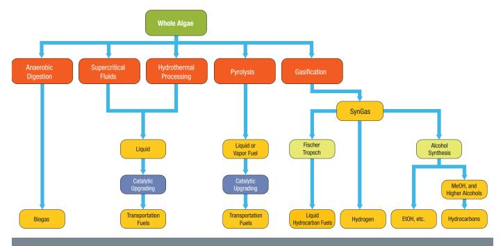
Figure 7.1. Schematic of the potential conversion routes for whole algae into biofuels (Source: Adapted from the 2010 National Algal Biofuels Technology Roadmap.)
