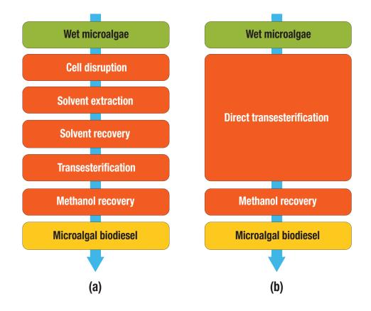
Figure 7.4. Chemical transesterification (a) and direct transesterification process (b) for production of biodiesel from algae (Source: Park et al. 2015)
