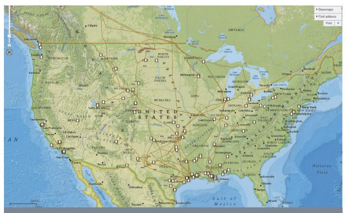
Figure 9.1. U.S. Energy Information Administration map of petroleum refineries, crude oil pipelines, and crude oil rail terminals (Source: EIA 2015)
