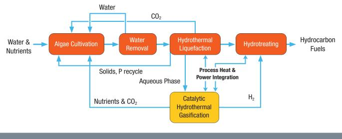
Figure 7.2. Hydrothermal processing of algae with nutrient recycle (Source: Elliott et al. 2015)
