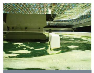
Figure 3.3. PNNL's indoor, LED-lighted, and temperaturecontrolled climate-simulation raceway pond (Photo courtesy of Michael Huesemann, PNNL)
