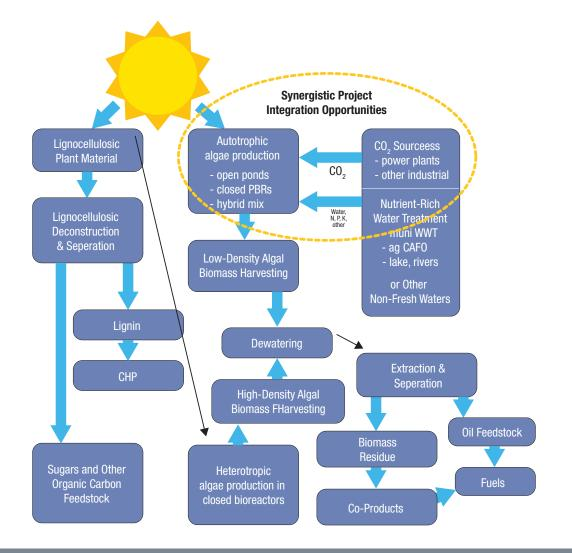
Figure 10.2. High-level illustration of heterotrophic and photoautotrophic approaches to microalgal biomass and biofuels production (Source: Adapted from the 2010 *National Algal Biofuels Technology Roadmap*.)
