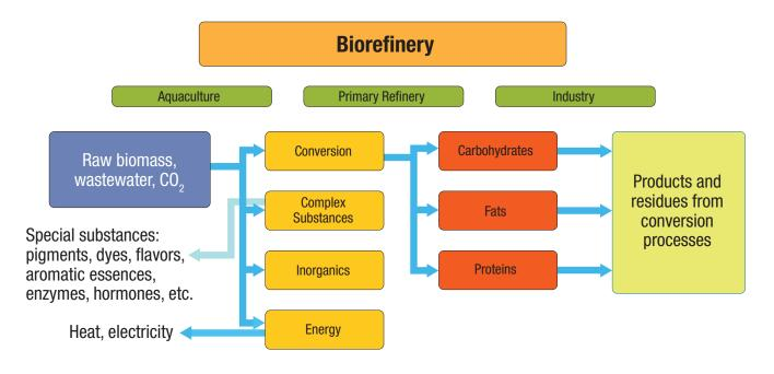
Figure 8.1. An overview of the biorefinery concept (Source: Modified from Kamm and Kamm 2007)
