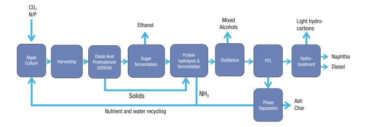
Figure 7.7. Process flow diagram for CAP coupled with protein fermentation (Courtesy of Ryan Davis, Sandia National Laboratories)
