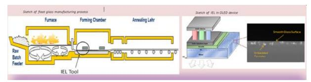
**Figure 6.26 IEL Layer Applied in a Float Glass Manufacturing Process** Source C.H. Hung, "Manufacturing Process for OLED Integrated Substrate," DOE SSL R&D Workshop Poster Session, Raleigh, NC, February 2016 [182]
