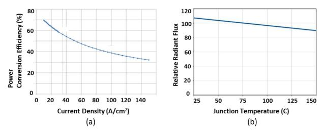
Figure 5.2 Two Types of Efficiency Droop: (a) Current Efficiency Droop, and (b) Thermal Efficiency Droop
