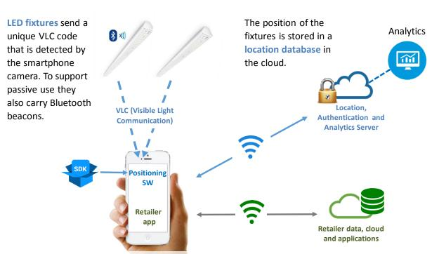
How light-based indoor positioning works
