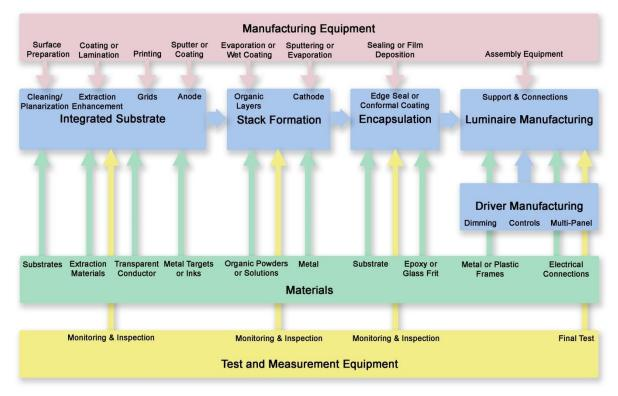
Note: The blue-shaded boxes and blue arrows describe the main manufacturing flow. The supporting elements of the supply chain are broken down into manufacturing equipment, materials, and test and measurement equipment. These supporting elements feed into the main manufacturing flow, as indicated by the relevant arrows.
