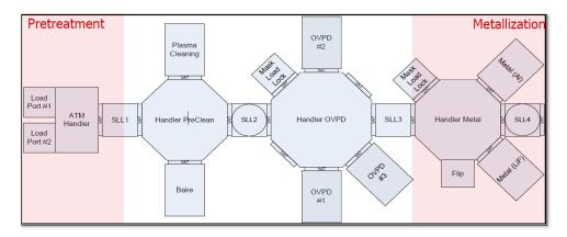
**Figure 6.30 Cluster Configuration for OLED Panel Manufacturing** Source: Juergen Kreis, Aixtron, OLEDs World Summit, San Diego, CA, 2016 [198]
