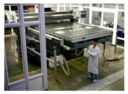
**Figure 6.27 InkJet Printing Platform for Gen 8 Substrates** Source: Kateeva Finally Unveils its Yieldjet OLED TV Inkjet Printing System [193]
