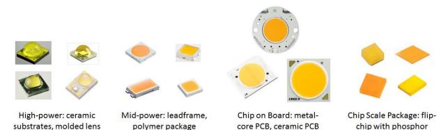
Figure 5.11 Examples of High-Power, Mid-Power, Chip-on-Board and Chip Scale LED Packages
