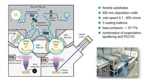
Figure 6.31 Prototype Line used at the Fraunhofer Institute FEP in Dresden Source: Christian May, Fraunhofer FEP, Smithers Apex OLEDs World Summit, Berkeley, CA, October 2015 [199]
