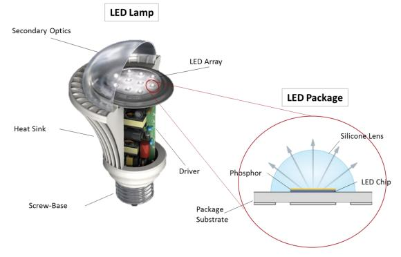
Figure 8.1 Components of an LED Lamp
