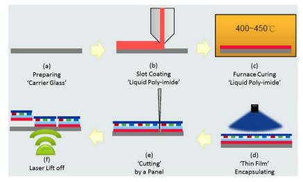
Figure 6.32 Use of Carrier Glass in Fabrication of OLED Panels on Plastic Substrates Source: David Hsieh, CIOS 2016 [214]
