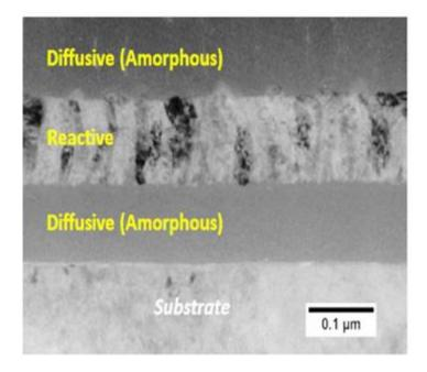
**Figure 6.25 Multi-Stack Barriers with Alternating Inorganic Layers of Varying Hardness (Vitriflex)** Source: Ravi Prasad, Vitriflex, "Transparent Barrier Films," OLED Stakeholder meeting, Pittsburgh, September 2015 [174]
