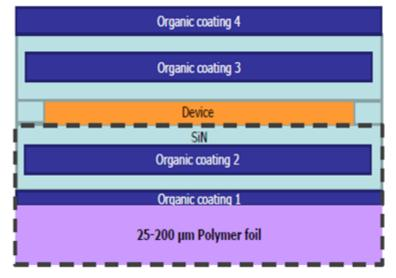
**Figure 6.22 Multi-Layer Barrier Coating to Prevent Ingress of Moisture and Oxygen** Source: Pim Groen, Holst Centre, DOE SSL R&D Workshop, San Francisco, CA, January 2015 [166]
