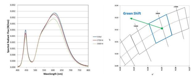
Figure 5.24 Accelerated Testing At 75°C and 75% Relative Humidity Shows a Shift in Red Phosphor Wavelength from 610 nm to 580 nm After 3500 hrs Resulting in an Overall Green Shift Source: Monica Hansen, Strategies in Light, Las Vegas, NV, February 2015 [94]
