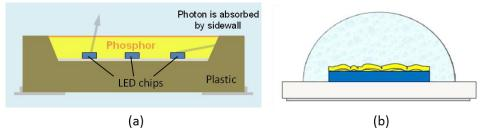
Figure 5.19 LED Package Schematics Showing (a) Sidewall Discoloration and (b) Phosphor Delamination
