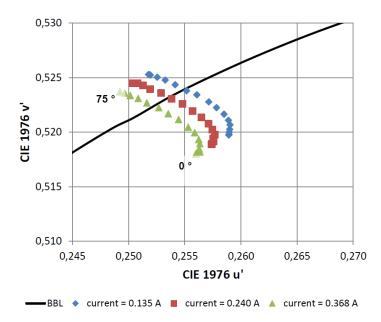
Figure 6.9 Variation of Color Point on CIE1976 (u',v') Diagram with Drive Current and Emission Angle Source: OLEDWorks FL300 Datasheet, 2016 [111]
