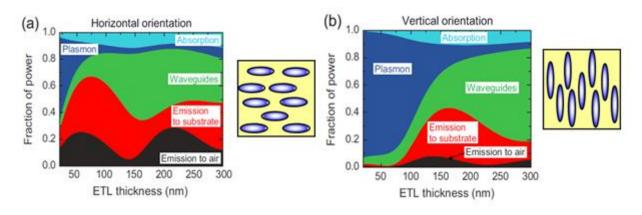
Figure 6.6 (a) Horizontally Oriented Emitters as Compared to (b) Vertically Oriented Emitters Source: B. Scholz et al, Optics Express Journal Entry, 2012 [133]
