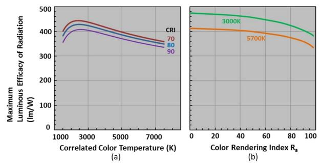
Figure 5.3 Theoretical Limits to White Light Luminous Efficacies of Radiation vs (a) CCT for a Given CRI, and (b) CRI for a Given CCT
