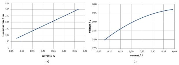
Figure 6.2 Dependence of (a) Luminous Flux and (b) Drive Voltage on Current Source: OLEDWorks FL300 Datasheet, 2016 [111]
