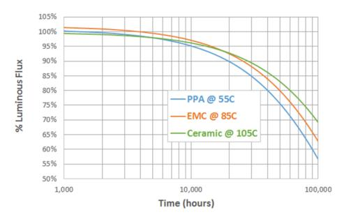
Figure 5.20 Lumen Degradation Performance of Typical Mid-Power Packages (PPA and EMC Plastic Resins) and High Power Packages (Ceramic Substrates). Source: Monica Hansen, Strategies in Light, Las Vegas, NV, February 2015 [94]
