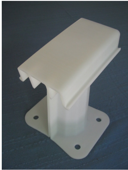
3-D printed (nylon) prototype of the FB-CC assembly.
