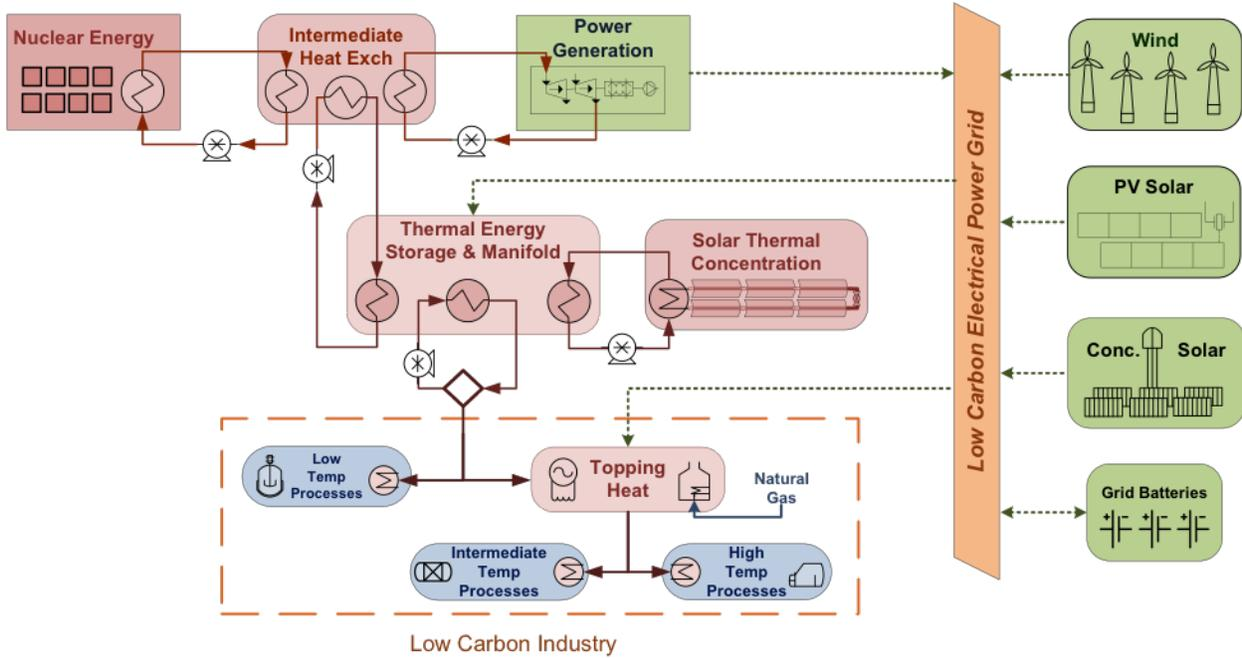
**Figure 4.K.3** General architecture for a loosely coupled (electricity only) nuclear renewable hybrid energy system, where the generation sources are only electrically connected to the industrial process. Note that electrical to thermal energy conversion systems may be included to provide thermal energy to some processes.
