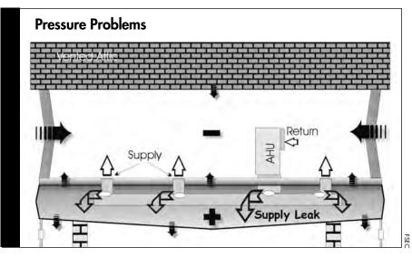
Figure 1. Supply leaks can cause positive pressures in the belly of manufactured homes. The resulting negative pressure in the living space can draw in moist air from the outside.
