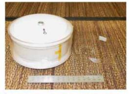
Coiled glass capacitor fabricated at Penn State by spraying Ag ink on the glass ribbon and then winding the ribbon around a mullite mandrel. Right side: free standing glass ribbon section Left side: fully packaged coiled glass capacitor
