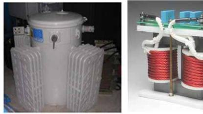
330kVA 60Hz Transformer250kVA 20kHz Transformer55" high and 2700Lb16" high and 75Lb
