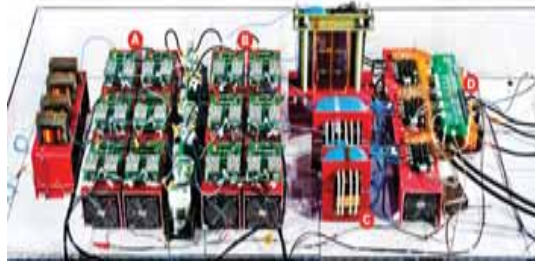
Gen- 1 SST: Si- based (3 kHz 6.5 kV IGBT)
