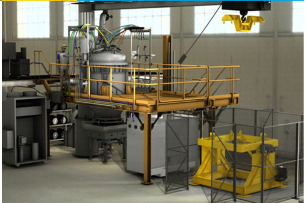
Large-scale bench reactor facility layout. Photo credit Berry Metal Company.
