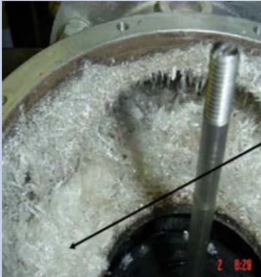
Crystallized light tars in IC engine intake manifold (courtesy Dahlman)
