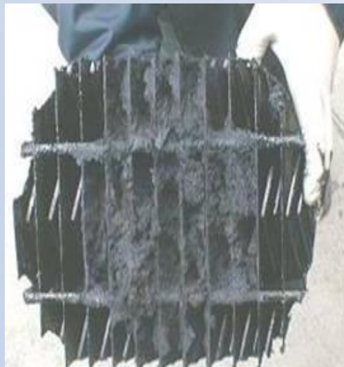
Heavy tar accumulation (courtesy ECN)
