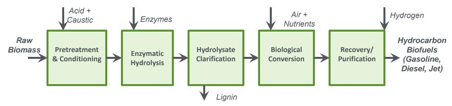
Biomass-derived sugars—separated from feedstocks through a series of chemical and biological processes—are further transformed, recovered, and purified to yield hydrocarbons for fuels and co-product commodities.
