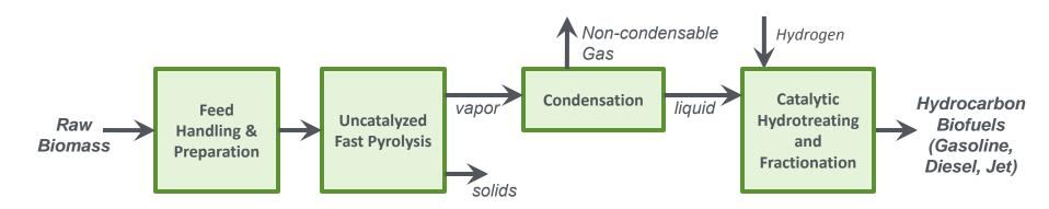
Biomass is rapidly heated in a fluidized bed reactor to yield vapors, which are condensed into a liquid bio-oil. This bio-oil is subsequently hydroprocessed to produce hydrocarbon biofuel blendstocks.
