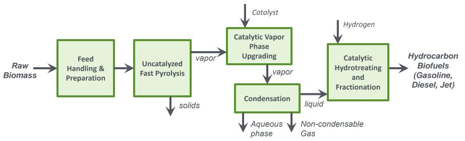
Biomass is rapidly heated in a fluidized bed reactor containing a catalyst to yield vapors, which are catalytically modified and condensed into a partially stabilized and deoxygenated liquid bio-oil. This stable bio-oil is subsequently upgraded to produce hydrocarbon biofuel blendstocks.
