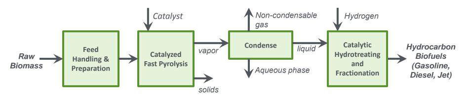
Biomass is rapidly heated in a fluidized bed reactor containing a catalyst to yield a partially stabilized and deoxygenated bio-oil vapor. The vapor is condensed into a liquid bio-oil and subsequently upgraded to produce hydrocarbon biofuel blendstocks.
