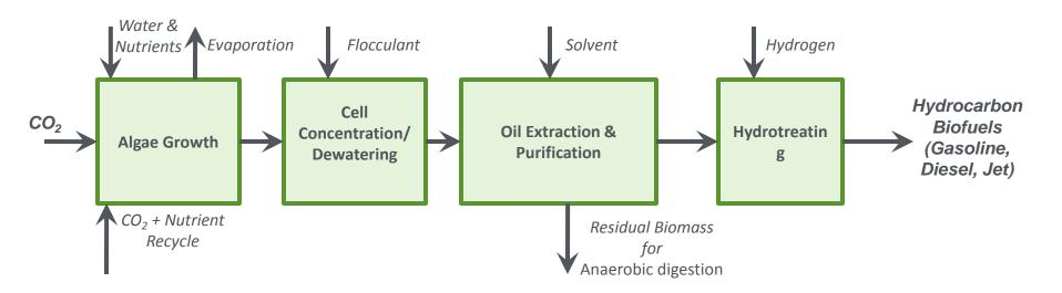
Lipids are extracted from wet algal biomass via high-pressure homogenization and a hexane solvent; the algal oil can then be hydrotreated to produce advanced hydrocarbon fuels.
