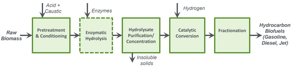
Biomass-derived sugars—separated from feedstock through a series of chemical and biochemical processes—are upgraded via aqueous phase reforming into hydrocarbons for fuels and co-product commodities.
