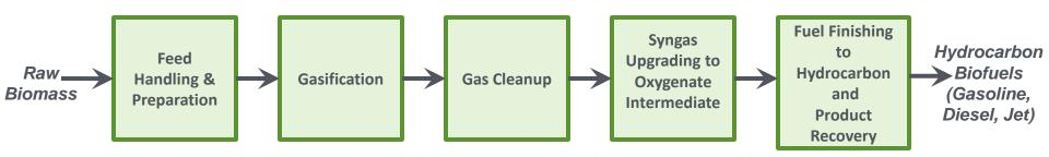
Biomass feedstocks are gasified to produce a clean syngas, which is used as a feedstock for hydrocarbon biofuel production.
