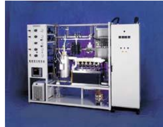
Laboratory scale reactor to evaluate catalyst performance and regenerability
