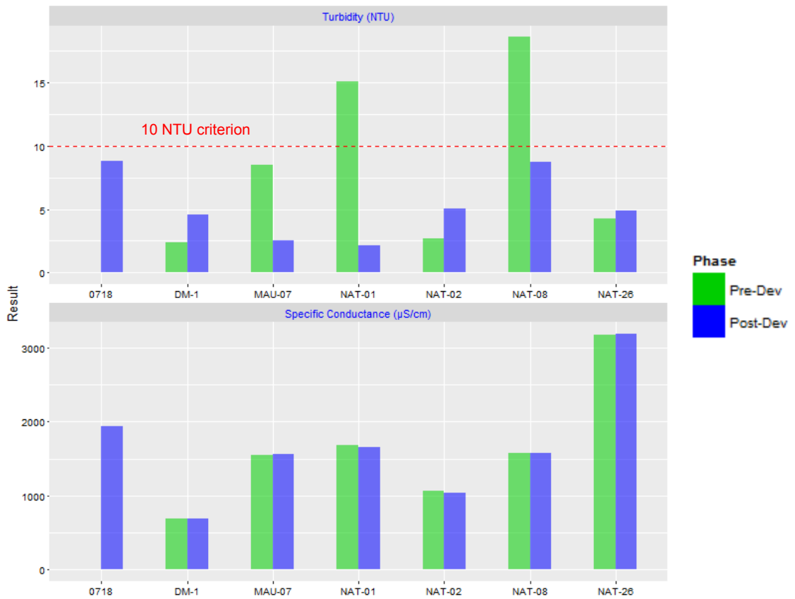
Figure 34. Pre- and Post-Redevelopment Turbidity and SC in Naturita Processing Site Wells Pre-redevelopment measurements were not taken at downgradient-most well 0718.
