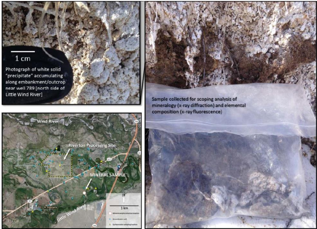
Figure 16. Riverton, Wyoming, Site Evaporite Mineral Deposits Top left and right, photographs of white evaporite mineral deposits observed along the escarpment at an abandoned oxbow channel of the Little Wind River. Bottom left shows the location of photographs and sample collection.
