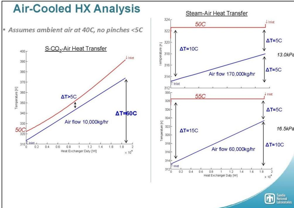
**Figure 3. Comparison of sCO<sub>2</sub> Brayton Cycle Effectiveness vs. Steam Cycle [24]**
