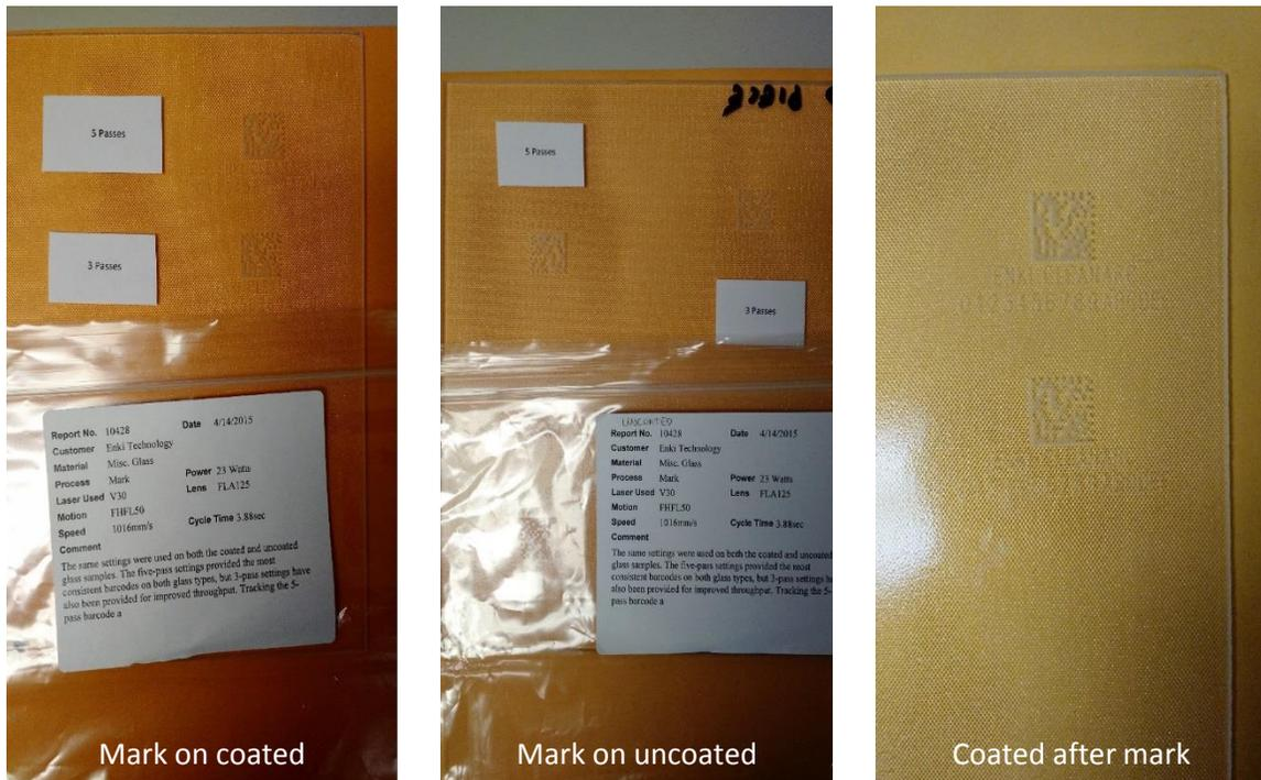
Figure 5 – Laser marked glass coupons
