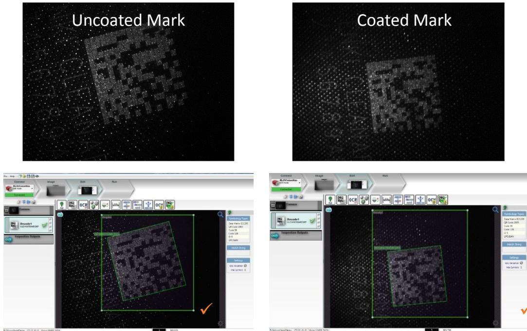
Figure 6 – Results of Barcode Reader Test
