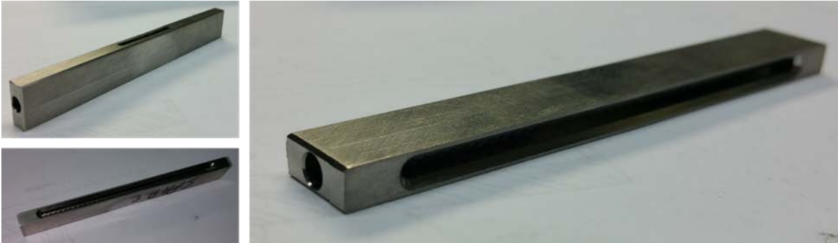
Figure 79 – Prototype header machined from IN625 plate stock.
