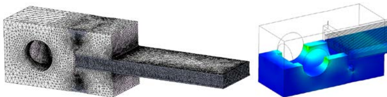
Figure 62 – FEA model of the fully assembled cell, header sleeve block, and header end-cap block. The model mesh is shown on the left, and stress contours are shown in cutaway on the right.
