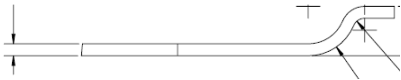
Figure 78 – Typical panel profile is a 2 dimensional bend and lends well to high throughput form or brake operations
