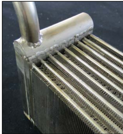
Figure 64 – Full heat exchanger core assembly, showing multiple manifolded cells welded together and capped with a semicircular flow channel. A single fluidic connection is welded to the semicircular flow channel.
