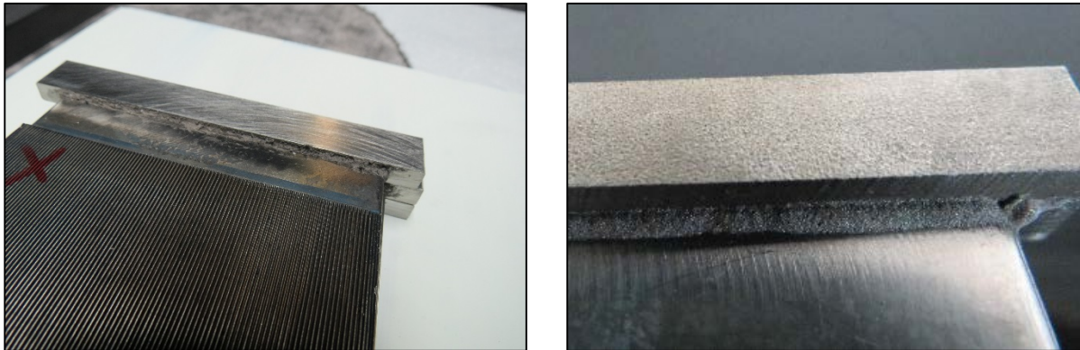
Figure 82 – Header sleeve being fit on a cell (left), braze alloy detail applied to back of header sleeve (right).
