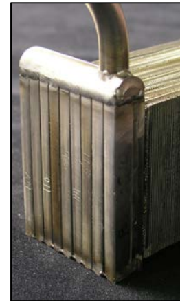
Figure 65 – Assembled core consisting of multiple cell subassemblies welded together at the manifolds and capped with a flow channel and connection.
