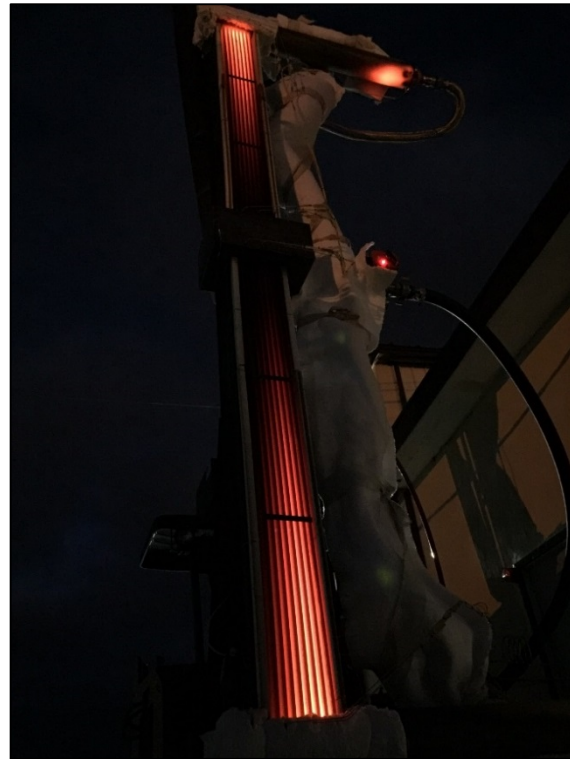
Figure 45 – The quartz window test section operating at night. Note the desired temperature gradient – wherein the peak temperatures are at the top and bottom manifolds – may be seen clearly.
