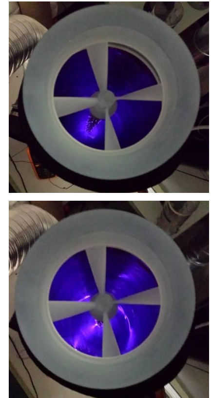
Downward view into GE precipitator while energized. Top photo 25KV, bottom photo 27.5KV
