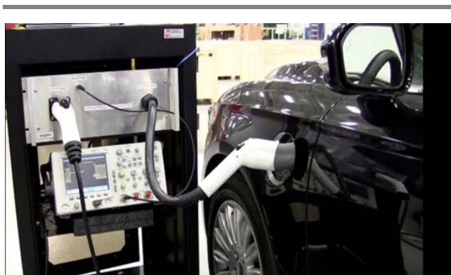
Figure 1. Testing data collection setup for one vehicle and EVSE pair.
