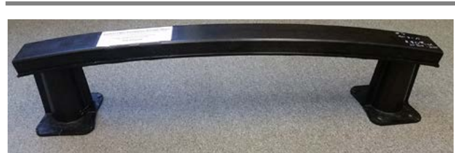
Figure 1. Carbon fiber FBCC, made from two compression-molded crush cans and a thermoset carbon fiber bumper beam with fabric C-channel and carbon SMC ribs.
