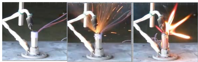
Figure 2. Left to right: A Li-ion cell with ISC device, a few minutes after melting the wax, and going into thermal runaway.
