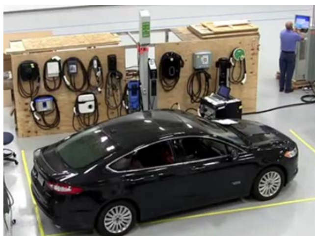
Figure 2. Testing area, and the EVSE and one vehicle in testing.
