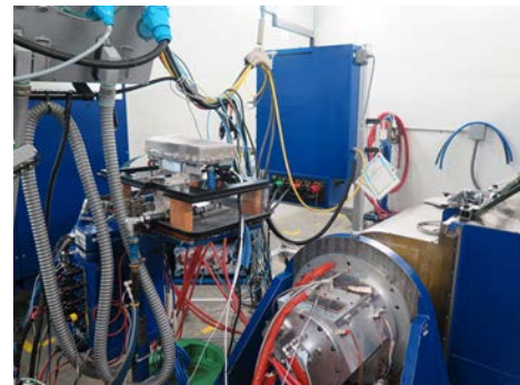
Figure 2. Then next-generation inverter prototype under active load test in GM's dynamometer laboratory.
