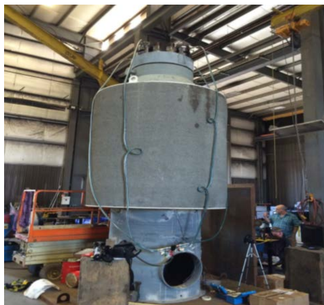
Figure 1. The low-cost steel concrete composite hydrogen storage vessel ORNL developed.
