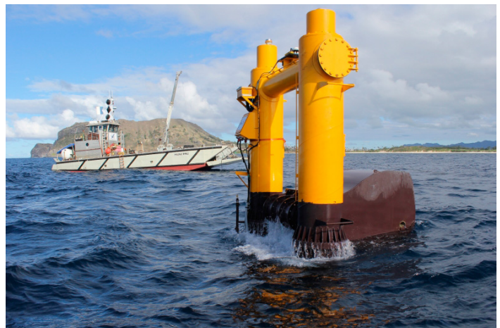
Energy Department-supported “Azura” wave energy converter is installed at a U.S. Navy test site in Hawaii. Photo courtesy of Northwest Energy Innovations.
