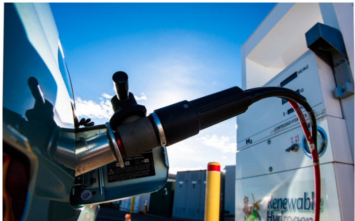
A fuel cell electric vehicle is refueled with hydrogen at the National Renewable Energy Laboratory’s National Wind Technology Center in Colorado. The H2 Refuel H-Prize is challenging America’s innovators to develop systems that make it easier and more convenient to fuel hydrogen vehicles. Photo by Dennis Schroeder, NREL
