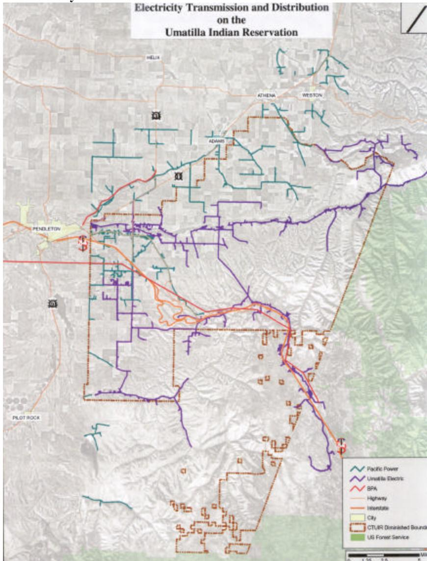
BPA has a 35 Mile 230 kV line crossing the Reservation in a 100 foot wide right of way. This line is a regional transmission line that runs roughly east-west through the UIR. A long term agreement between the CTUIR and BPA has been established to accommodate this line.
