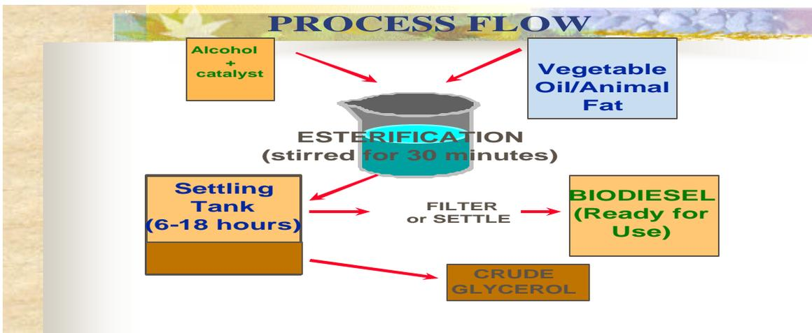
Figure IV 3.2. Small-Scale Biodiesel Production Using Cruzesterification Process.
