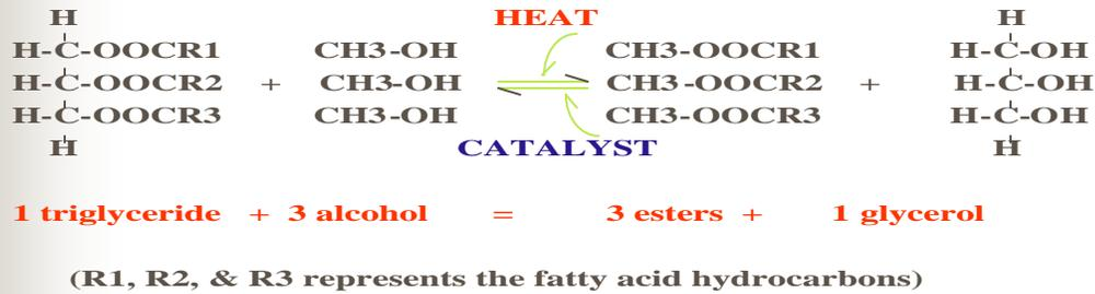
Figure IV 3.1. Transesterification Process to Produce Biodiesel.
