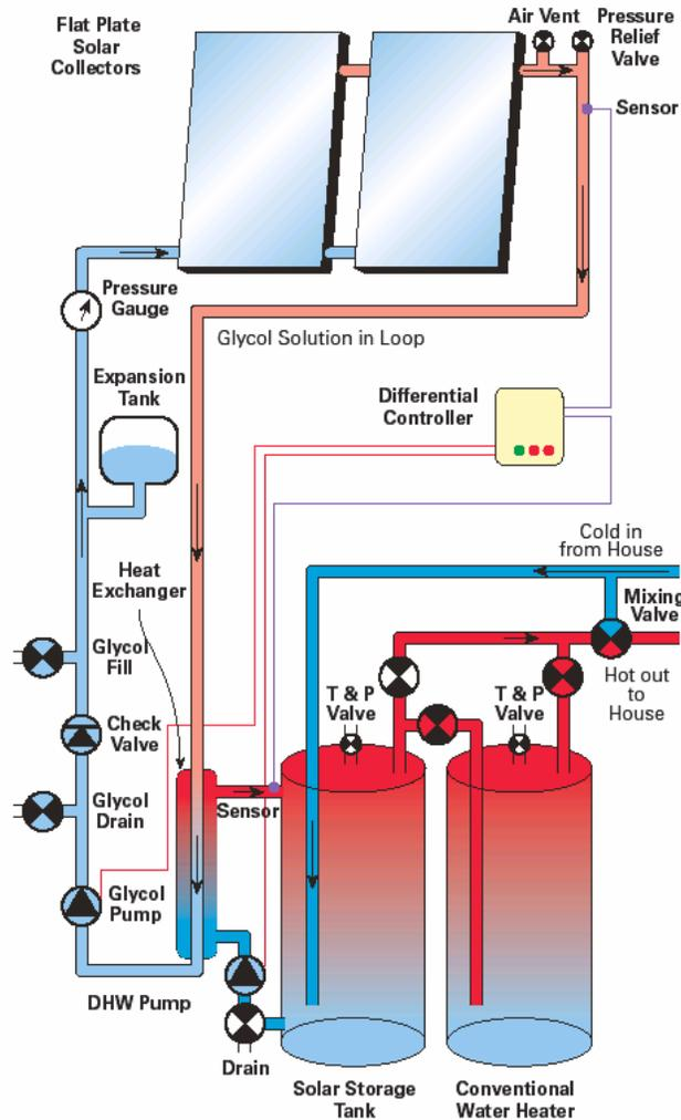
Figure IV-5-5 Parts of a typical solar domestic hot water system
