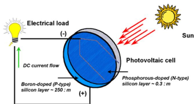
Figure IV-5-7 Diagram of a photovoltaic cell
