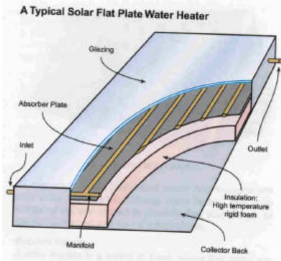
Figure IV-5-4. A flat plate solar collector for producing domestic hot water
