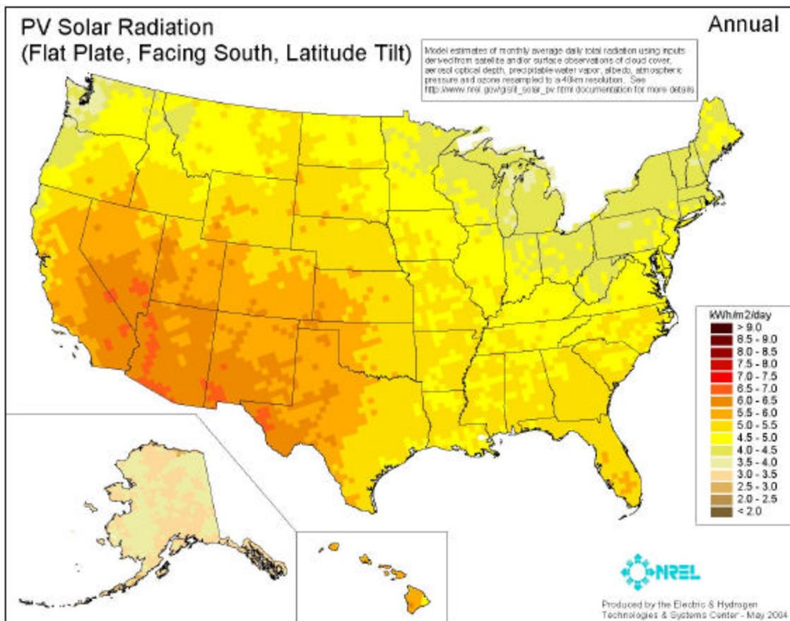
**Figure IV-5-1** Average annual solar radiation assuming fixed, flat plate collectors, facing south, and tilted with the latitude. From the National Renewable Energy Laboratory web site.
