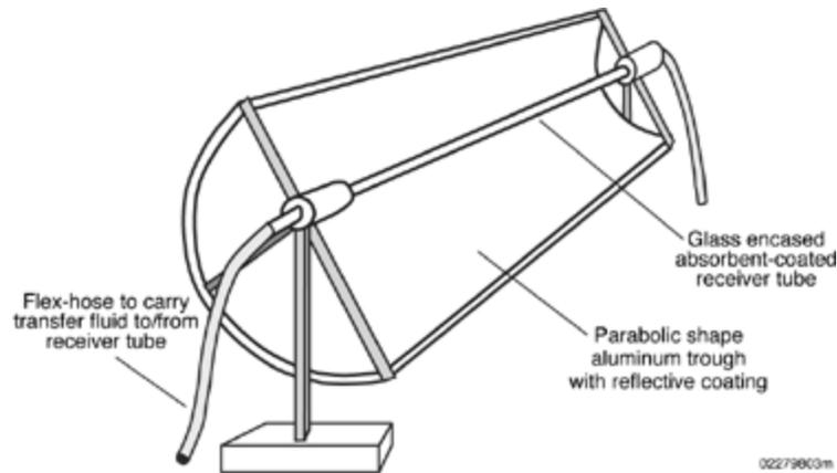
**Figure IV-5-6 A concentrating solar reflector for producing hot water for domestic or commercial use.**
