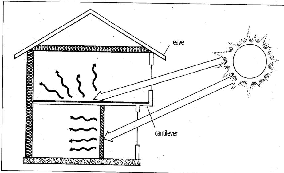
**Figure IV-5-3. A passive solar home with overhangs to shade in the summer but allow sun in during the winter. A thermal mass slowly re-radiates the sun's energy during the night.**
