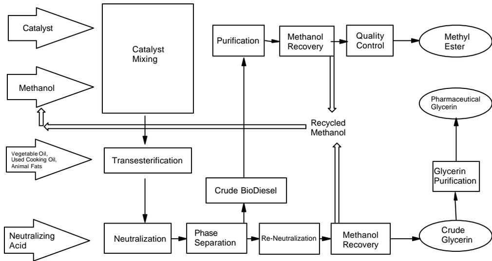
Figure IV.3.43 Commercial Biodiesel Process Schematic
