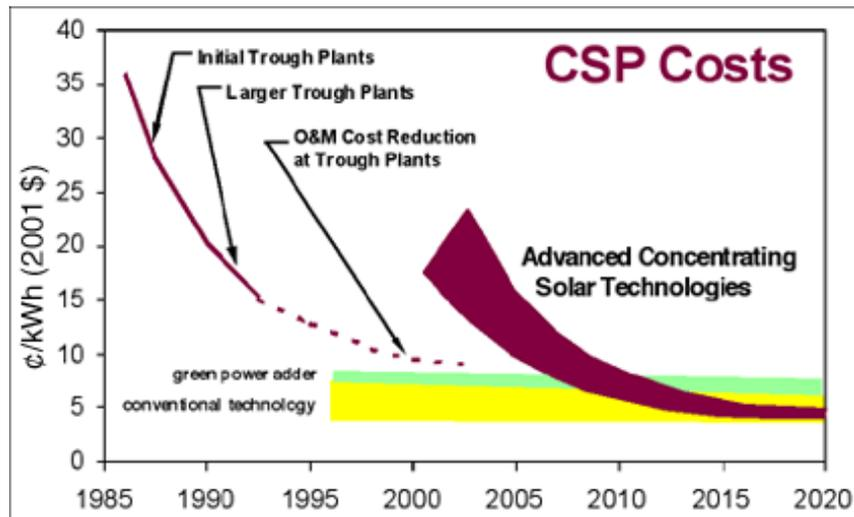
Figure IV-5-10 Concentrating Solar Projected Costs
