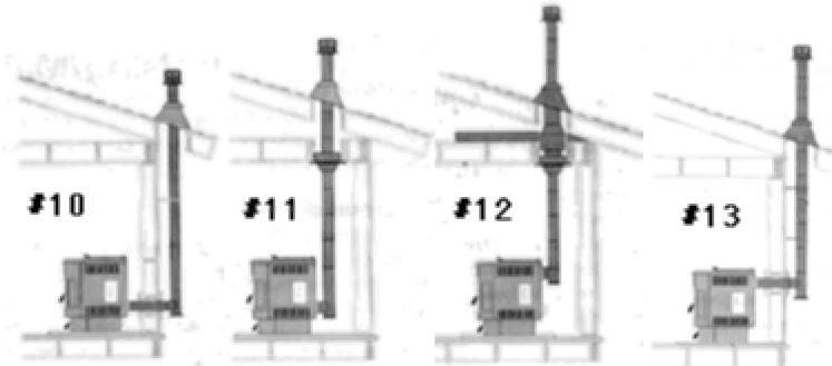
Vertical (Figure 12) extends up from the stove and penetrates the ceiling and roof. Horizontal and vertical (Figure 13). Extends from the top or back of the appliance, penetrates the wall, turns up to penetrate the eave and roof. Venting into existing chimney (see Figure 8). Follow manufacturer's recommendations for venting into masonry and factory-built chimneys, which may include partial or full chimney relining.
