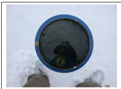
Pathfinder Reading Taken on Casino Roof Top
