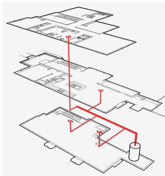
The standard domestic water heating packages offered at Stapleton include a conventional trunk-and-branch piping arrangement. In the sample home, the builder placed the water heater at one end of the basement, and hot water fixtures are spread out over the two floors above. The system has considerable piping length and excessive stored water volume between the domestic water heater (DWH) and the fixtures. An isometric diagram of the pipe to the most remote fixtures is shown at left.
