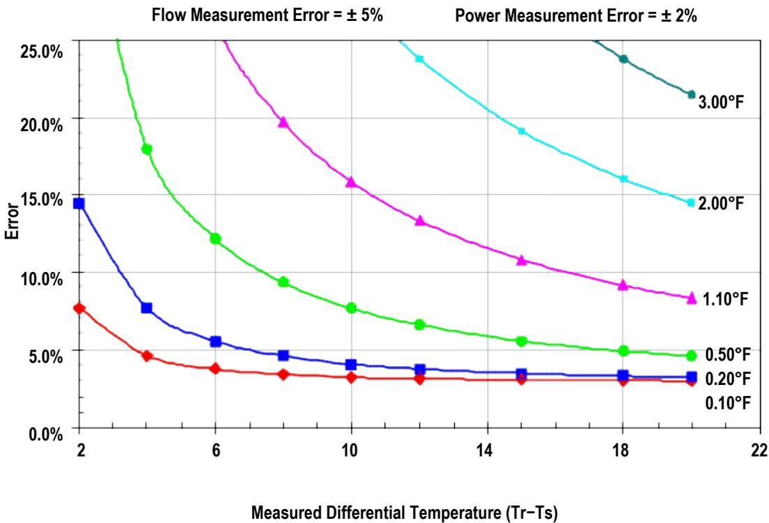
**Figure 5-2. Example Influence of Sensor Accuracy on Calculations.<sup>23</sup>**
