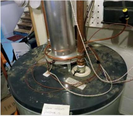
Instrumented water heater at a field-test site
