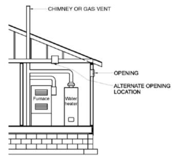
1 sq in/3,000 Btu/hr input Not less than sum of vent connectors
