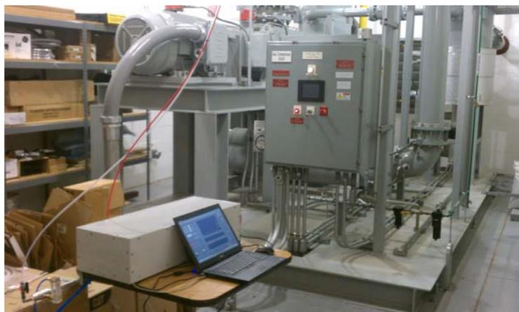
A gas quality sensor (GQS) setup at Bath Landfill, Steuben County, NY. Real-time GQS technology and engine control system improvements are addressing fuel quality issues with opportunity fuels such as landfill gas and digester gas.
