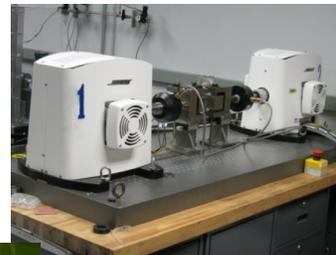
Used fuel rod stiffness experiments and analyses
