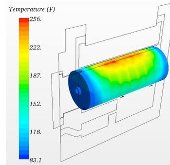
*CFD Thermal Analysis of Dry Storage Casks
