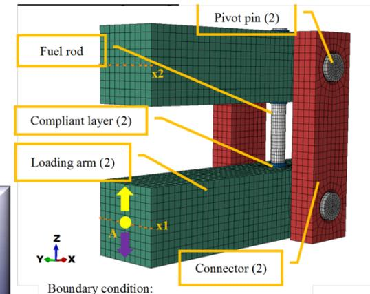
*FE Model of Rod Bend Tests
