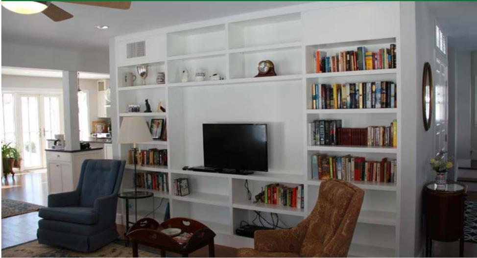
High-efficiency ducted heat pumps are installed in central locations on the first and second floors to provide heating and cooling through very short duct runs that are located within the home's conditioned space. A first-floor supply register is visible here above the book case. The second-floor ducts are located in a ceiling cavity between the drywall ceiling and a plywood attic floor.
