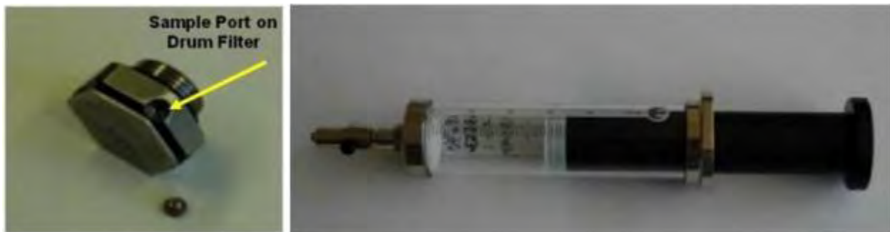
Figure 6-45: Syringe to Pull Gas from Drum or SWB via Sample Port on Filter
