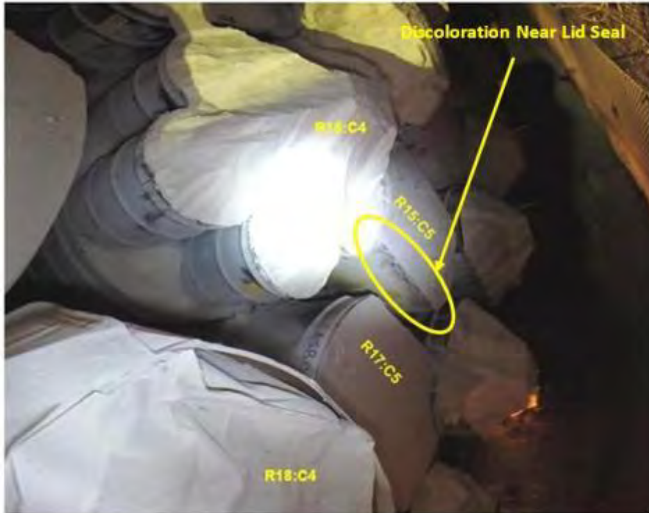
Figure 6-35: Discoloration of SWB at R15:C5
