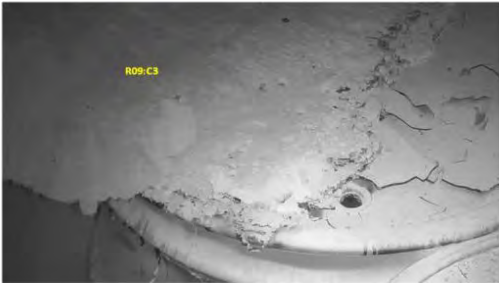
Figure 6-19: Residual Polyethylene on Dunnage Drum at R09:C3
