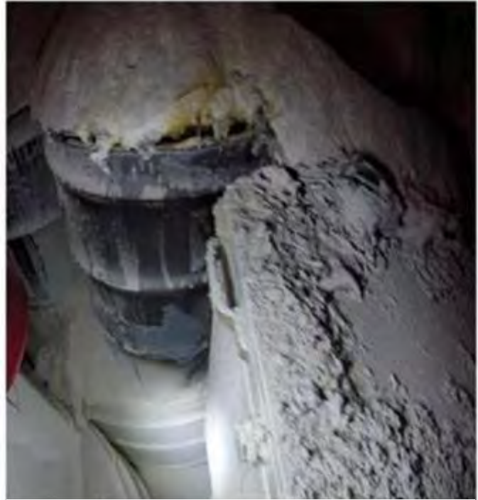
Figure 2-3: Drum 68860 Lid Failure
