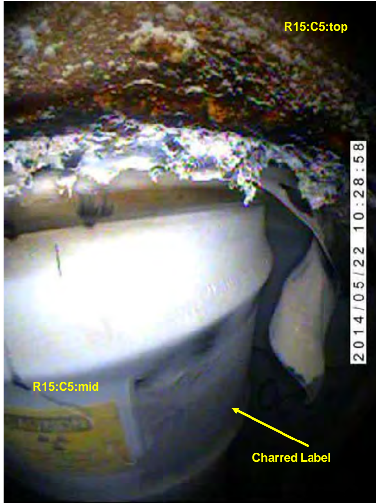
Figure 6-39: Charred Label at R15:C5
