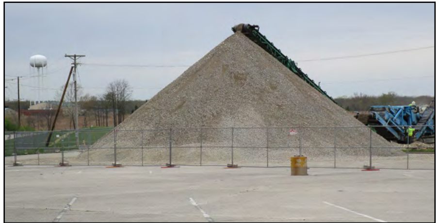
Rock crushing operations produced 2,157 cubic yards of gravel.
