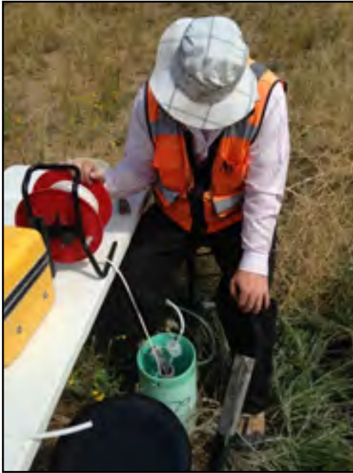
Scientist measuring specific conductance at an LM site monitoring well as part of the Variation Project.
