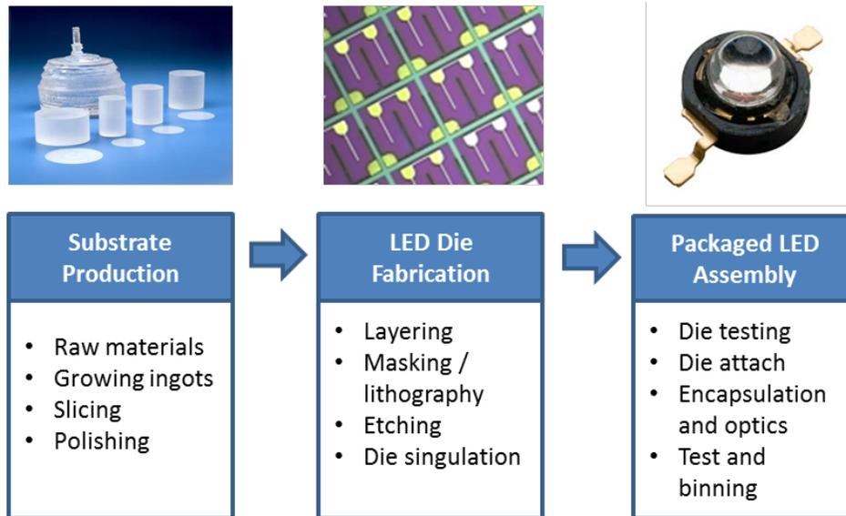
**Figure 5-1. Three Major Stages of Packaged LED Manufacturing**
