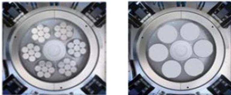
**Figure 4-2. Comparison of MOCVD Reactor Tray, 2” versus 6” wafers**
