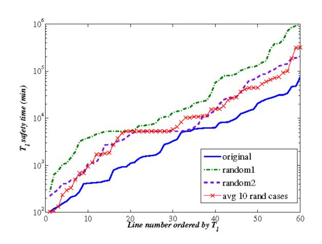
IEEE-300 bus system, given the same topology, G/L/C ratios, and generation and load statistical settings, the test cases with random bus type assignments tend to have larger expected safety time than that of the realistic grid settings.
