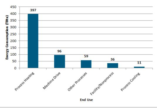
Figure 2-7. Steam Consumption in the Petroleum Refining Sector by End Use, 2010 (DOE 2014)
