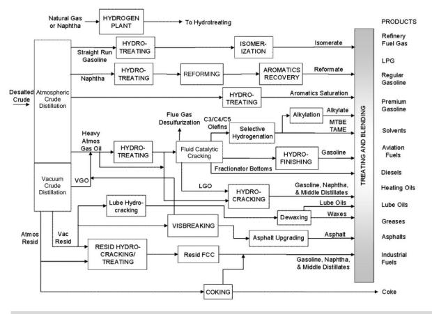
Figure 2-2. Typical Petroleum Refinery Flow Diagram (DOE 2007)
