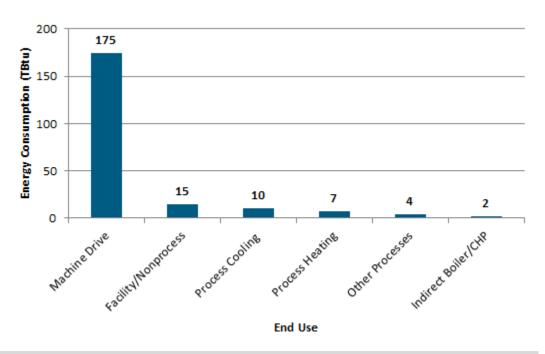
Figure 2-6. Electricity Consumption in the Petroleum Refining Sector by End Use, 2010 (DOE 2014)
