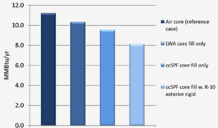
A simple ccSPF core fill reduced basement zone heat loss by 15%. Combining a ccSPF core fill with R-10 exterior rigid insulation installed to 1 ft below grade reduced heat loss by 27%.
