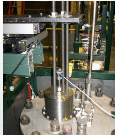
**Figure 4. Experimental setup with a bellows mounting assembly of a UWT.**
